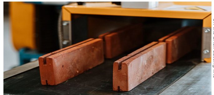
Cut and grooved slips coming off the brick cutting line
