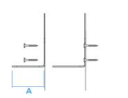
For cavity barriers 76mm-90mm wide (across cavity) use 2 MP brackets and the 65mm long spike (A).
