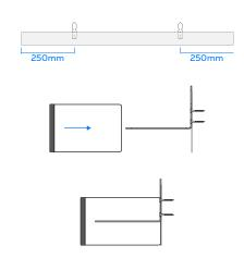
VFB Plus - Product width across cavity from 91mm up to 215mm fixed using 2 multi purpose (MP) 160mm brackets.
