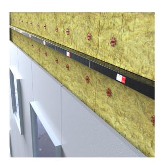
VFB 120/120- Product width across cavity 16mm up to 75mm wide, directly faced fixed, no additional pigtails required.
