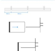
Fix 3 number MP brackets, per linear meter, to the substrate at maximum 150mm from the end of the cavity barrier, with a maximum spacing between brackets of 350mm.
