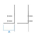
For cavity barriers 76mm-90mm wide (across cavity) use 2 MP brackets and the 65mm (A) long spike.
