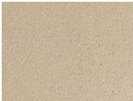
FL ferro light sandblasted at low pressure, rough surface
