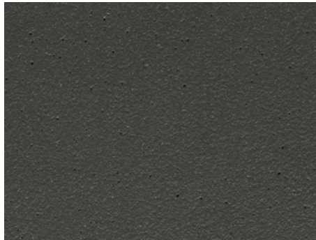
FL ferro light sandblasted at low pressure, rough surface
